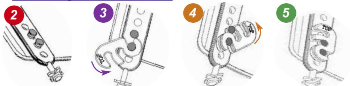
A hingelock consists of a two part **Prong** and **'S' clip**. Remember no tools - fingers and hands are all that's needed.
